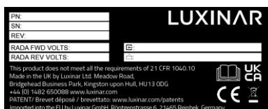
Figure 11 - Label A1.8 — RF power supply product identification
